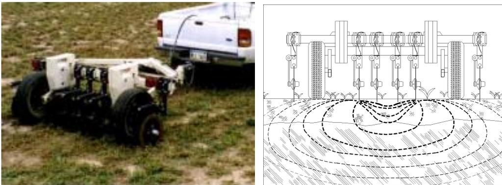
**Figure 1.** Veris Technologies 3100 soil EC mapping systems; signal array shown at right.
