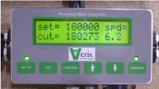
Veris PosiRate™ technology includes planting rate motor output shown on the cab console
