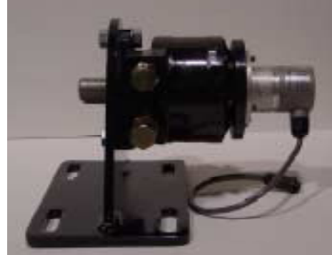
Here's why Veris drives are so smooth—a high resolution encoder and a large displacement motor running at low rpm.
